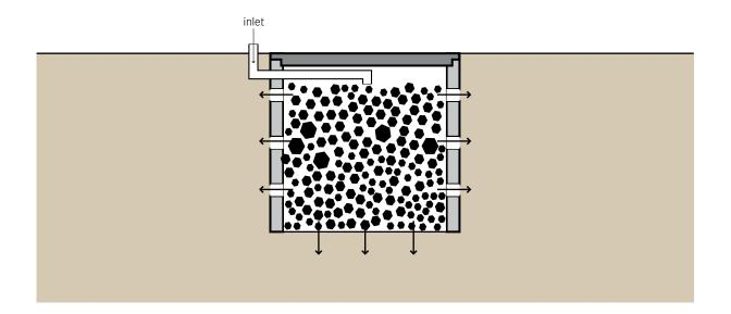
A soak pit, also known as a soakaway or leach pit, is a covered, porous-walled chamber that allows water to slowly soak into the ground. Pre-settled effluent from a Collection and Storage/Treatment or (Semi-) Centralized Treatment technology is discharged to the underground chamber from which it infiltrates into the surrounding soil.
